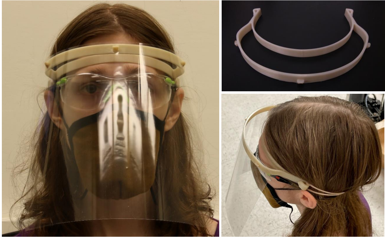
Figure 6: A researcher wearing a face shield 3D printed from CoPA. After autoclaving face shields printed from CoPA there is only a small amount of deformation, and the part remains fully usable.
