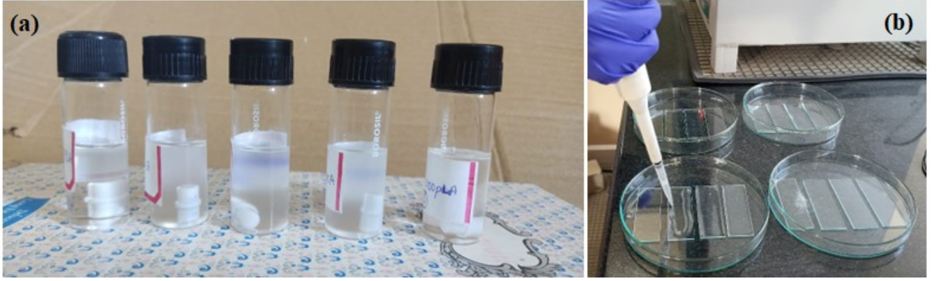
FIG. 1: (a) Variation of P(VDF-TrFE):PLA blend composition, left bottle contains 0:100 (pure PLA), 25:75, 50:50, 75:25, and the right bottle contains 100:0 (pure P(VDF-TrFE)); (b) Casting technique adapted in film making.
