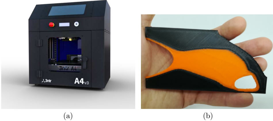
Figure 5: FDM machine at ProtoLab and 3D printed cantilever beam
